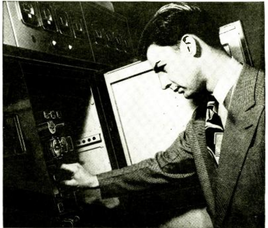
Author checks frequency on built-in scope at WCTS, Cincinnati. Motor control is above hand.
