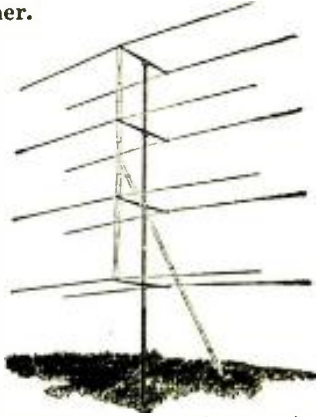
Fig. 6—A sensitive and directional antenna.
